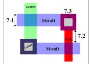
SCMOS Layout Rules - Via Vias must be drawn orthogonal to the grid of the layout. Non-Manhattan vias are not allowed.
