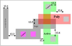
Exceptions for AMIS C30 0.35 micron process: <sup>1</sup> Use lambda=4 for rule 12.2 only when using SCN4ME <sup>2</sup> Use lambda=4 for rule 12.2 only when using SCN4ME\_SUBM
